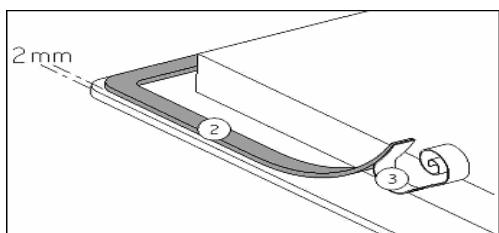
Stick the gasket (2) two millimetres from the external edge of the glass, after removing the protection tape (3).
