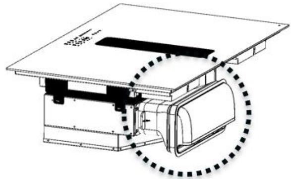
For cutting the opening for the extraction duct through the cabinet, please refer to the provided template.
