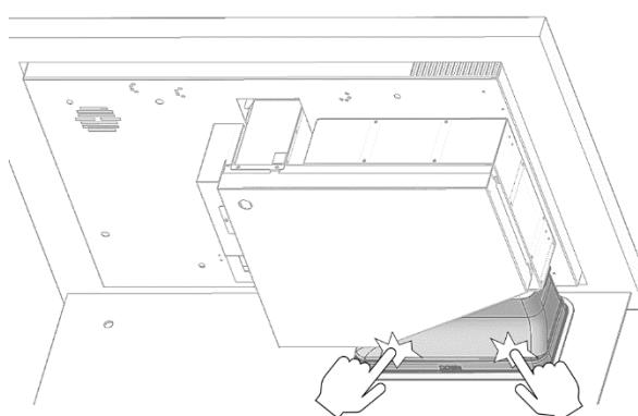
Once the table and the extraction duct are in place inside the cabinet, press the duct against the rear of the cabinet to ensure a tight fit.
