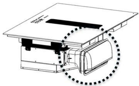
For cutting the opening for the extraction duct through the cabinet, please refer to the provided template.
